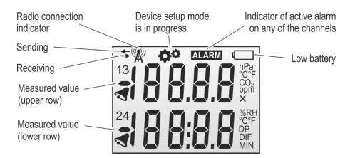
Radio Connection Indicator – indicates successful activation of the device in the LoRaWAN® network. If the device is within range of the network, the indicator lights up approx. 15 s after switching on the device and remains lit. The indicator starts flashing if no radio message from the network arrives to the device for more than 23 h. If this state lasts longer than 48 h, the indicator will go off, indicating a probable loss of connection to the network.
