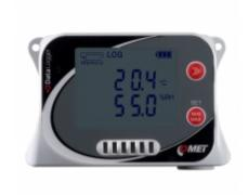
Datalogger is designed to record temperature and humidity. The recording is performed in a non-volatile electronic memory. The data can be transferred to a PC via USB-C.
