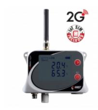
GSM Datalogger is designed to record temperature from two external Pt1000 probes. In case of exceeded set limits, SMS and JSON messages can be sent via GPRS data connection. Measured values can be sent to the internet storage <a href="COMET Cloud">COMET Cloud</a>, which is a complete monitoring, alarm and analysis system.
