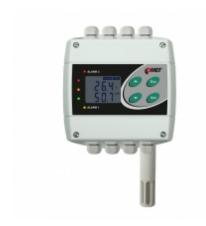
Humidistat, thermostat with two relay outputs. Outdoor, indoor use. Built-in relative humidity, temperature sensors. Measured values are also converted to other humidity interpretation: dew point temperature, absolute humidity, specific humidity, mixing ratio, specific enthalpy. Three two-state inputs.
